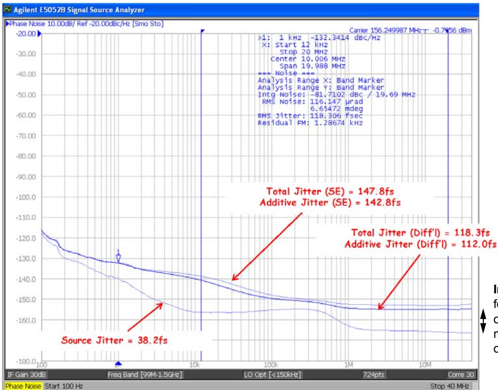
Figure 13. Source Jitter (156.25 MHz)
