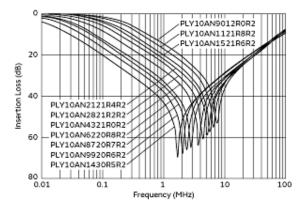
Differential Mode Insertion Loss (Typ.)
