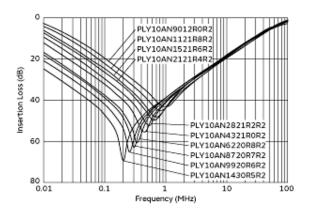
Common Mode Insertion Loss (Typ.)
