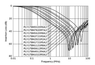
Common Mode Insertion Loss-Frequency Characteristics
