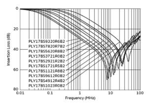
Common Mode Insertion Loss-Frequency Characteristics
