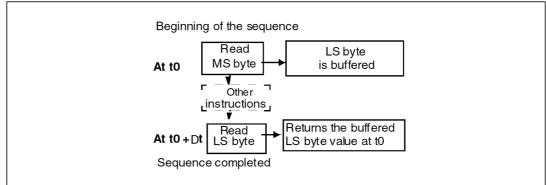
Figure 1. 16-bit read sequence for the counter (TIMx\_CNTR)
