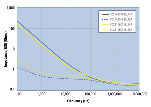
The measurements were taken at room temperature (25°C)
