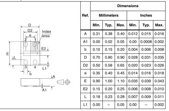
Figure 14. Footprint dimensions (in mm) Figure 15. Marking
