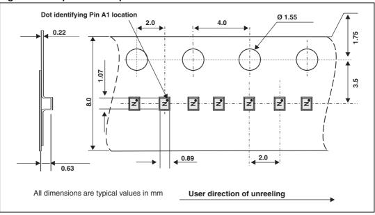
Figure 16. Tape and reel specifications
