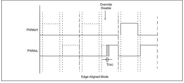
In Complementary Output mode, the expected dead time between transitions of the PWMxH and PWMxL outputs may not be asserted when the following occurs:
