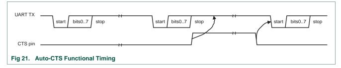
While starting transmission of the initial character, the  $\overline{\text{CTS}}$  signal is asserted. Transmission will stall as soon as the pending transmission has completed. The UART will continue transmitting a 1 bit as long as  $\overline{\text{CTS}}$  is de-asserted (high). As soon as  $\overline{\text{CTS}}$  gets de-asserted, transmission resumes and a start bit is sent followed by the data bits of the next character.
