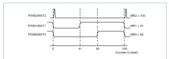
Fig 49. Sample PWM waveforms with a PWM cycle length of 100 (selected by MR3) and MAT3:0 enabled as PWM outputs by the PWCON register.
