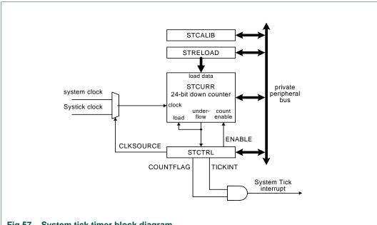
Fig 57. System tick timer block diagram
