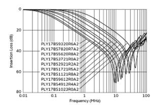
Common Mode Insertion Loss-Frequency Characteristics
